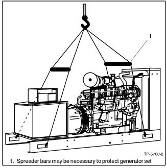
Figure 2-2 Generator Set with Lifting Hooks in Skid
